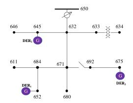
Fig. 3. The modified IEEE 13-node distribution system
