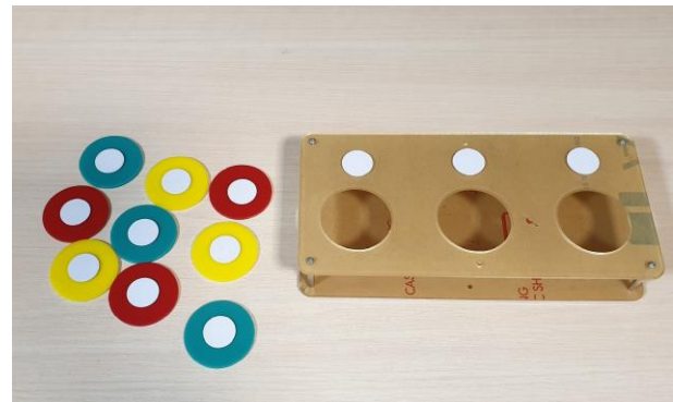
Fig. 4: Setup 2. Nine circular disks with different colors were used along with one box with three holes of the same size. Each circular disk and hole had an RFID tag attached to them.
