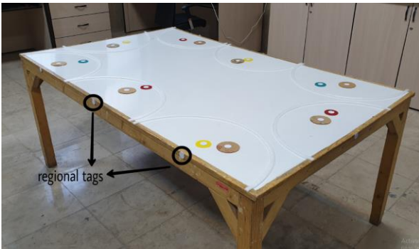
Fig. 6: Setup 4. A rectangular table was divided up into 8 sections, labeled with RFID tags by alphabet characters. There are two or three disks inside each region.
