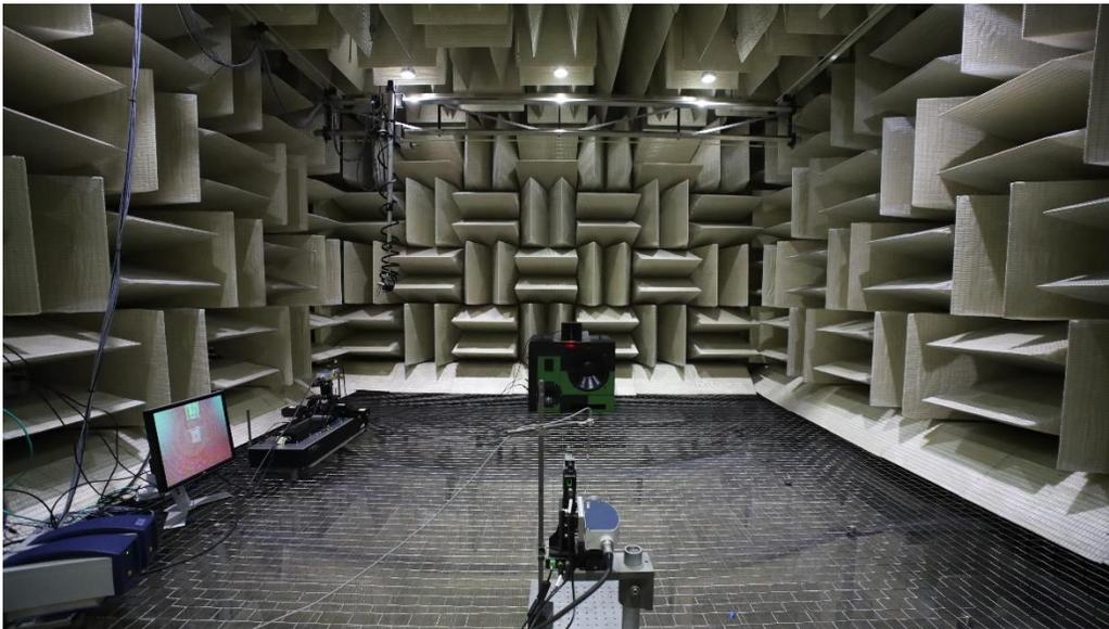
Fig. 1 Anechoic chamber at Binghamton University
