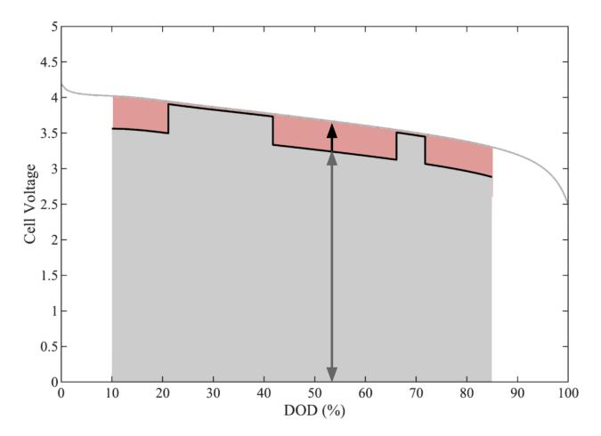
Here the black discharge curve is the discharge profile for our example vehicle introduced in Part 5. The discharge energy required to complete the mission is the area in grey. The area under the corresponding portion of the OCV curve includes the pink and grey areas.
