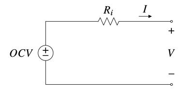
The potential across the voltage source is the cell's open circuit voltage and the resistance is the cell's internal resistance. Both the OCV and the Ri are functions of the cell depth of discharge -- they depend on where you are in a cell's discharge.
