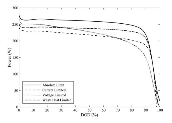
Thinking in terms of an aircraft, there will be some minimum power required of the cells late in the mission. While this may simply be to maintain cruise flight, it likely involves a higher power requirement such as aborting a landing or arresting the descent in a vertical landing.
