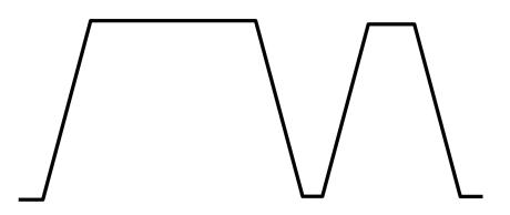
This mission includes a primary segment followed by a reserve mission requiring a divert. Each segment is made up of a takeoff, cruise, and landing segment. Each segment is specified in terms of time and power level as given below.
