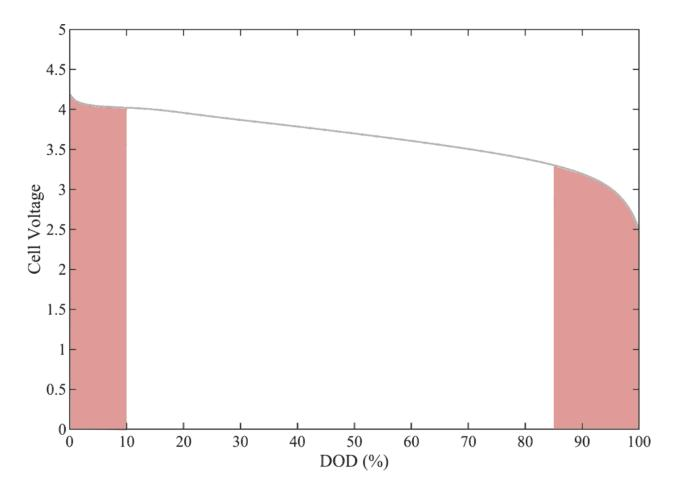
For mental calculations, we can assume that each portion of charge contains equal energy, allowing us to approximate the partial energy knockdown as the usable charge fraction.
