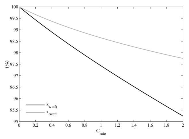
The premature cutoff effect mentioned earlier is illustrated by the grey curve in this figure. This effect is neglected by the simple approximation provided by the prior equation.
