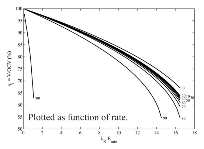
The fact that the curves were remarkably flat in the prior figure leads to the lines for different depth of discharge nearly collapsing in this figure.
