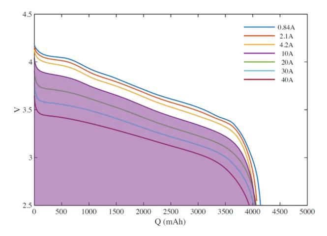
In order to zoom in on the interesting part of the chart, the vertical axis of discharge rate maps usually does not go to zero, so be careful about visually comparing areas under the curves -- there is often more area off the chart than on.
