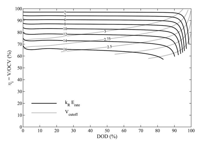
In this figure, additional grey lines are included to illustrate the effect of the cell cutoff voltage -- the minimum voltage power limit. Other power limits could be plotted in similar fashion.
