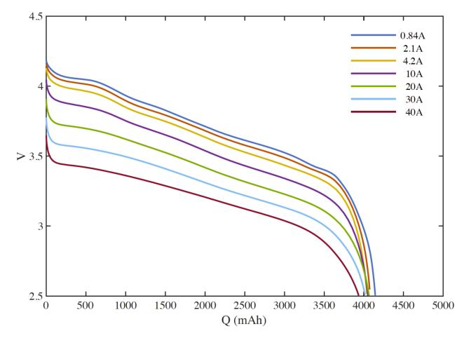
A rate map depicts the discharge voltage (vertical axis) as a function of cell capacity (horizontal axis) for different constant current discharges (each colored line).
