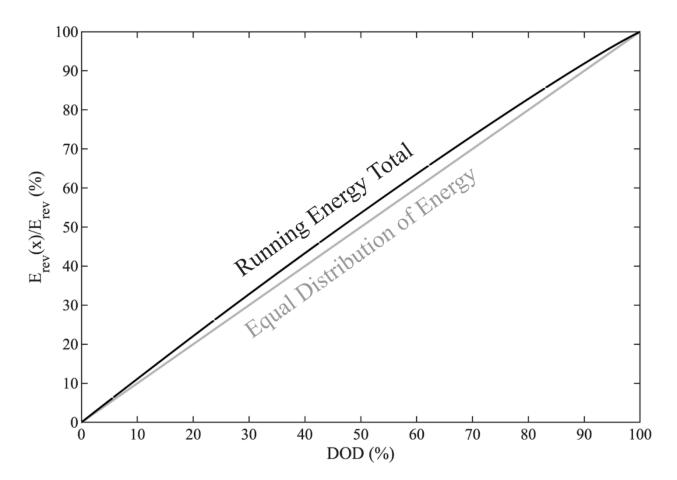
This curve starts out steeper than the equal distribution curve because the top of charge contains more energy per charge than the cell average.
