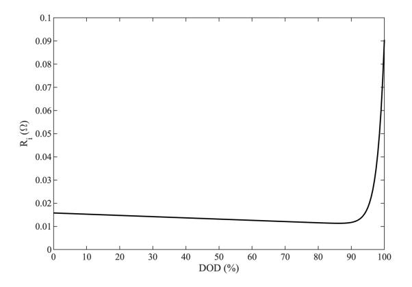
We will require OCV and Ri curves like those shown above. These may be provided by the cell manufacturer or they can be reverse engineered from a typical discharge rate map. Although there are theoretical means of predicting these curves, they are almost always empirically derived in practice. The functional form of these curves is irrelevant to our purposes, linear interpolation or functional fits to data are acceptable.
