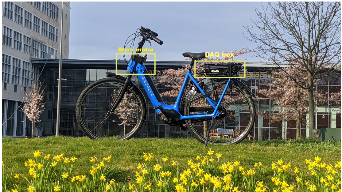
Figure 2. Second prototype Balance assist bicycle at Delft University of Technology in collaboration with Royal Dutch Gazelle and Bosch eBike Systems. The steer motor and the data acquisition box (DAQ) are annotated in the picture.
