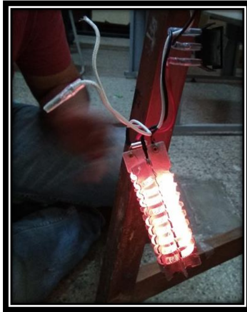
Figure 2 Hot air gun heating system
