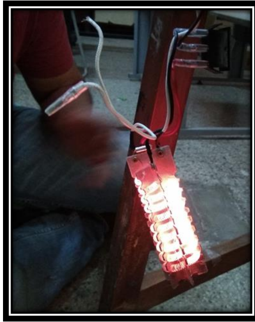
Figure 2 Hot air gun heating system
