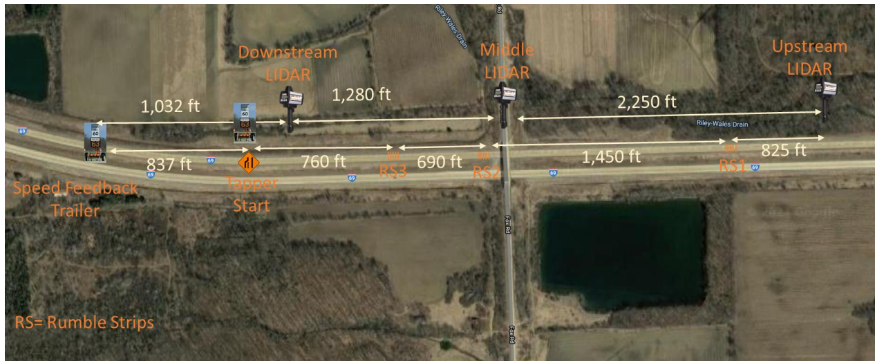
FIGURE 3. WB I-69 work zone and data collection setup
