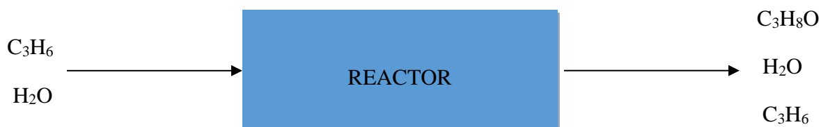
Figure 4.1 Reactor with inlet and outlet streams used in the manufacture of isopropyl alcohol 50 tons/day
