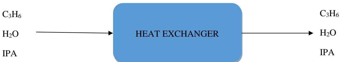
Figure 5.2 Heat exchanger with inlet and outlet streams used in the manufacture of isopropyl alcohol 50 tons/day
