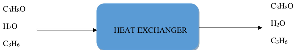
Figure 4.2 Heat Exchanger with inlet and outlet streams used in the manufacture of isopropyl alcohol 50 tons/day
