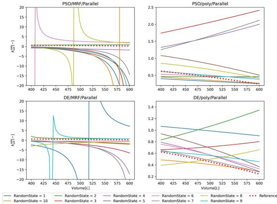
Figure 4: Profile of the  $k_{UA}^{HM}$  predicted with the parallel approach with the various combination of optimiser and black-box structure. MRF return poor prediction capabilities and low robustness since the numerical instabilities and wrong trend. The usage of the polynomial function returns better prediction capabilities than the MRF. In this case, when DE is used as the optimiser, the parameter estimation shows higher robustness with the initial population.
