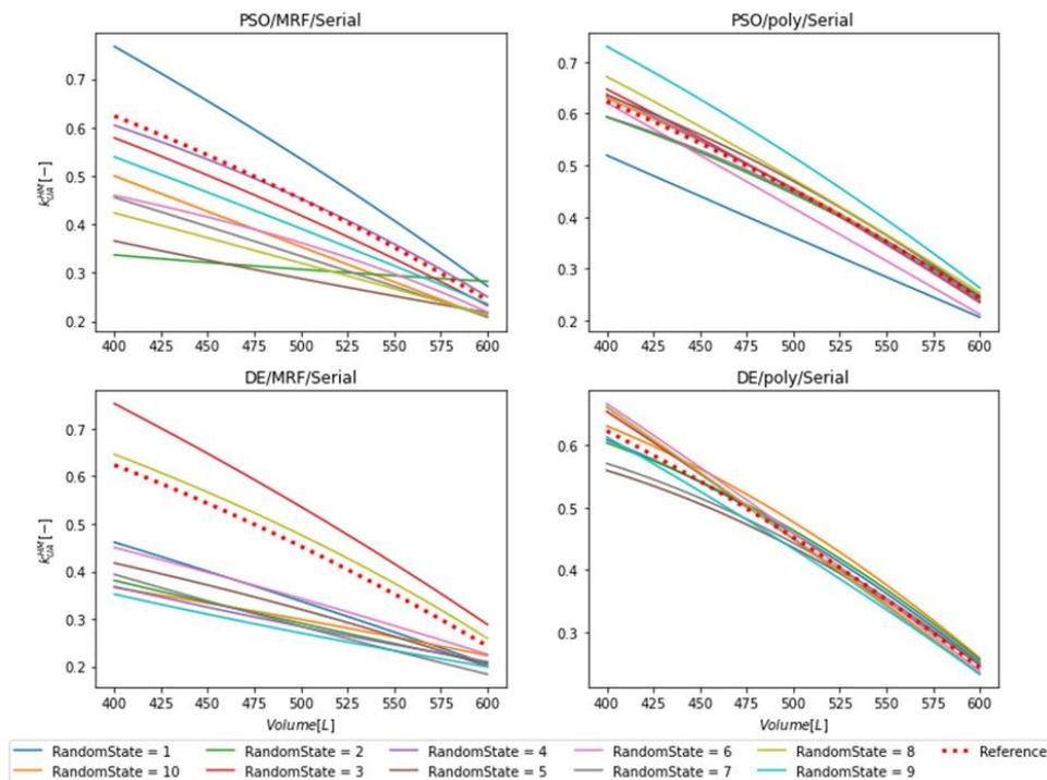
Figure 6: Predicted profile of  $k_{UA}^{HM}$  obtained with the serial approach with various combinations of optimisers and black-box structure. All the solutions are within the acceptable range and follow the correct trend of the predicted variables. However,
