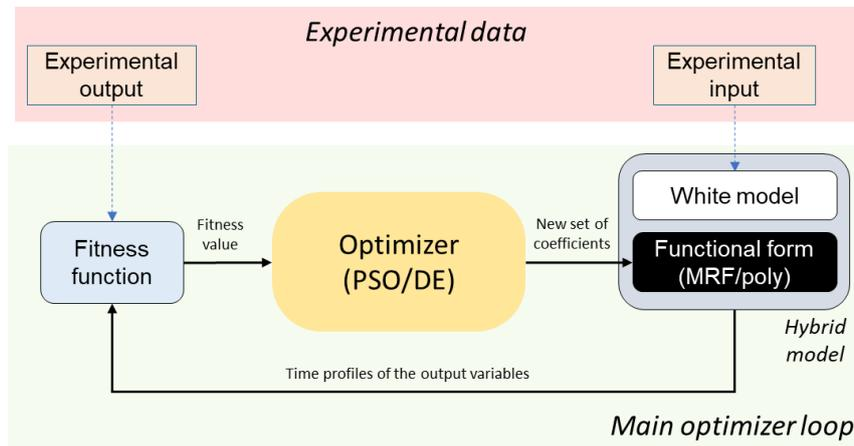
Figure 2: Hybrid model training structure. The coefficients set proposed by the optimiser is used to run the simulation driven by experimental input. The model returns the estimated time profile of the output variables. These are compared with the experimental output from the plant, and the fitness function is calculated using these deviations. The calculated value of the fitness function is given to the optimiser, which will propose a new set of coefficients to test.
