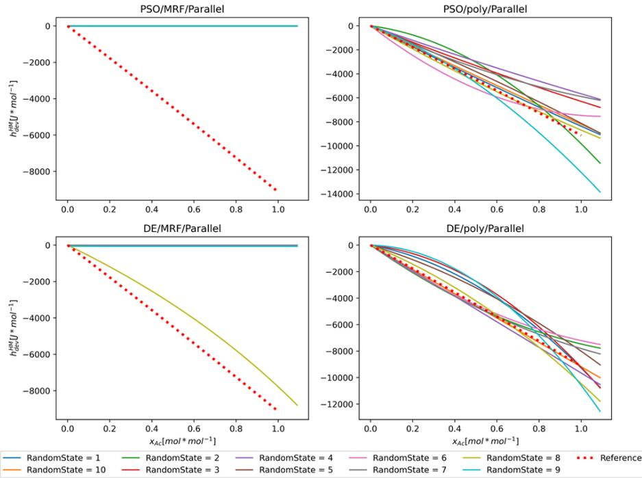
Figure 5: Profiles of the  $h_{dev}^{HM}$  predicted using the parallel approach with the various combination of optimiser and black-box structure calculated at 50°C. The polynomial functions show higher robustness and accuracy than the MRF. The models obtained with the MRF show numerical instabilities and poor accuracy regardless of the used optimiser. The polynomial function shows higher prediction accuracy and robustness with the random state with both the optimisers.
