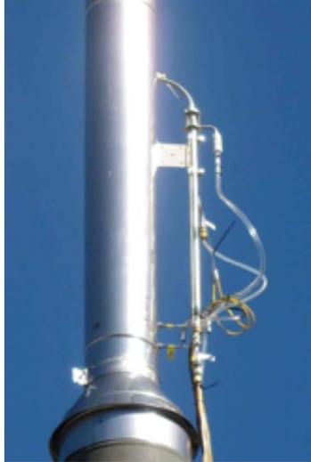
**Figure 3.** Flue extension and venturi diluter mounted to the outlet of wood heater chimney [59].
