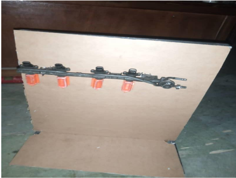
Figure 3.5: Injector Rail Mounted on the Frame
