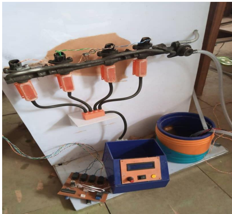
Figure 3.6 Connection of the ECU to the injector rail
