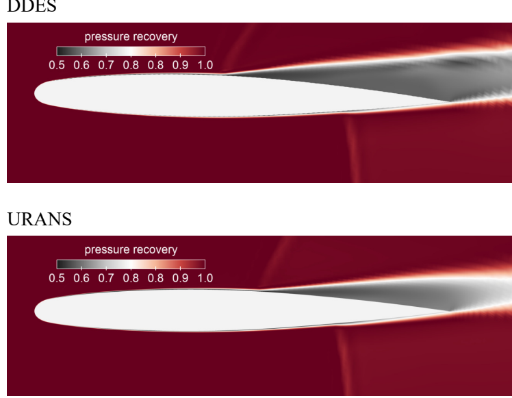
FIG. 20. Contours of the pressure recovery factor in the cutting plane at 90% of the wingspan, obtained from the simulation of the static deformation subjected to the flow at Ma = 0.925 and p_{dyn} = 215 \text{ kPa} .
