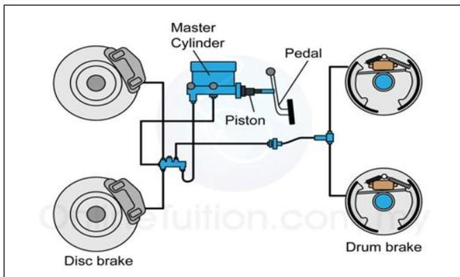
Figure 4.6.1 Hydraulic braking system
