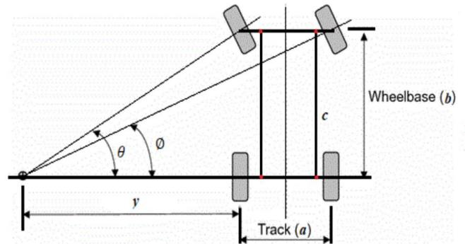
Figure 2.1 Ackermann steering mechanism
