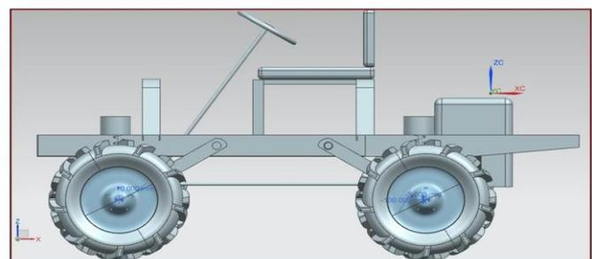
Figure 3.3 Left view of ATV – 4WS
