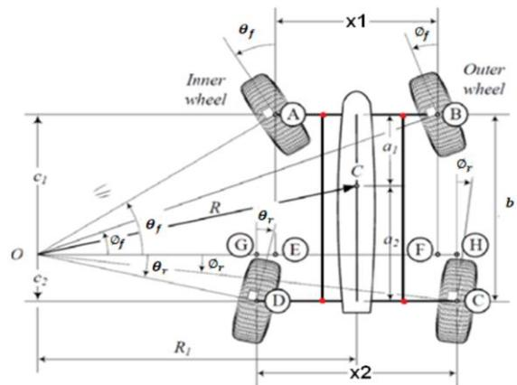
Figure 2.2 Correct Four wheel steering mechanism
