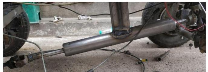
Figure 4.5.1 Transfer shaft developed.
