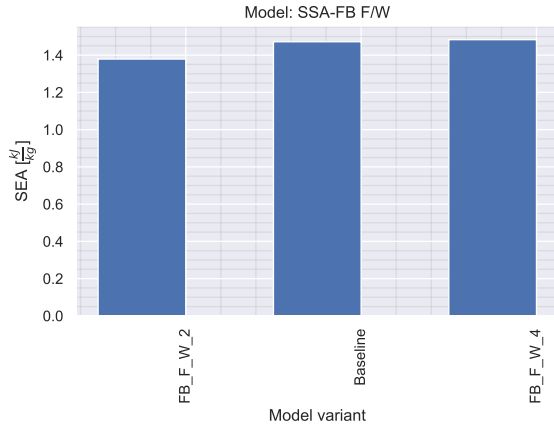
Fig. 17: SEA for cross beam height-to-width ratio sensitivity analysis. SEA only slightly increases for larger ratios since, when keeping flexural rigidity constant, the cross beam becomes lighter for higher ratios.
