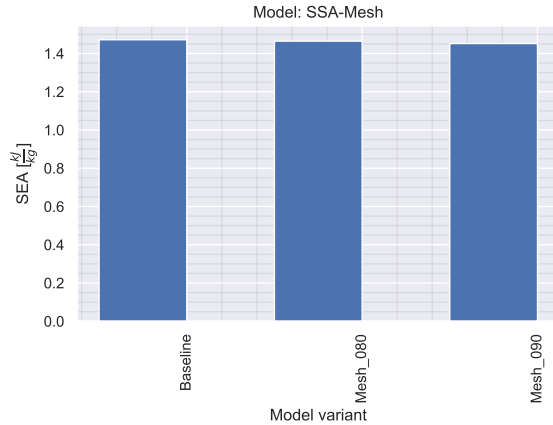
Fig. 13: SEA for mesh sensitivity analysis variants. All models have almost identical SEA.
