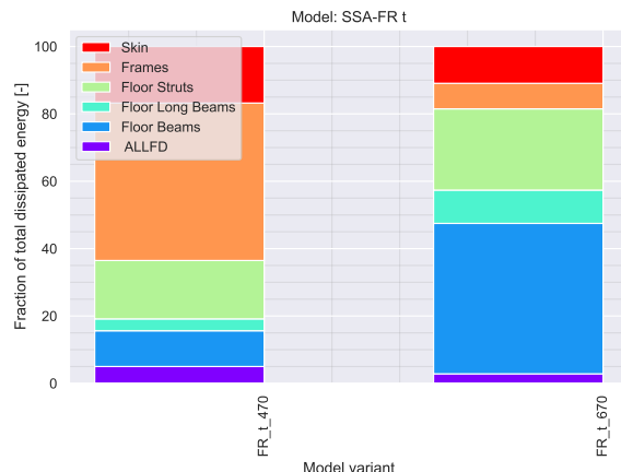
Fig. 25: Energy absorption distribution by component, frames thickness sensitivity analysis. The frames’ bending stiffness has a significant impact on the energy-absorption characteristics of the section.
