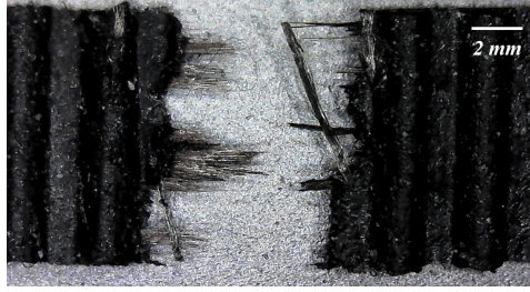
Figure 3: Belt break interface, showing broken fibers
