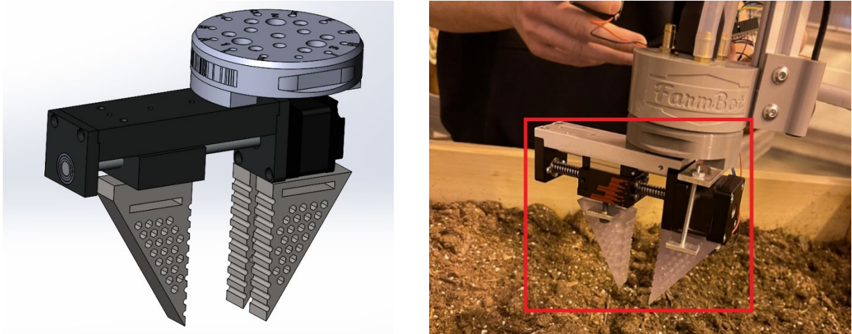
Figure 2. (left) A CAD rendering of a student designed gripper and (right) a fabricated prototype of the same gripper, with the student-designed portion highlighted by a red box.
