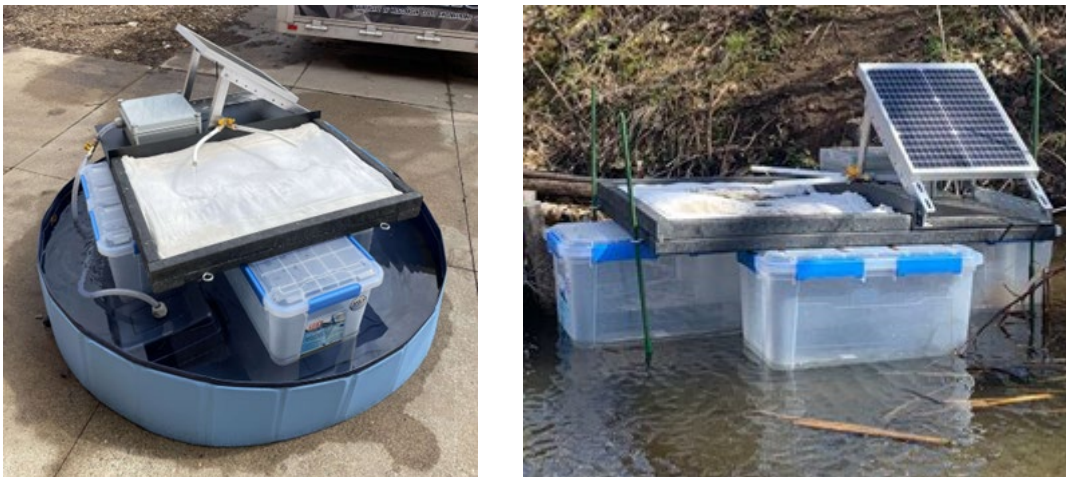
Figure 5. Final design prototype for a lake-sediment transporter (left) shown in a small pool and (right) shown deployed in a lake.
