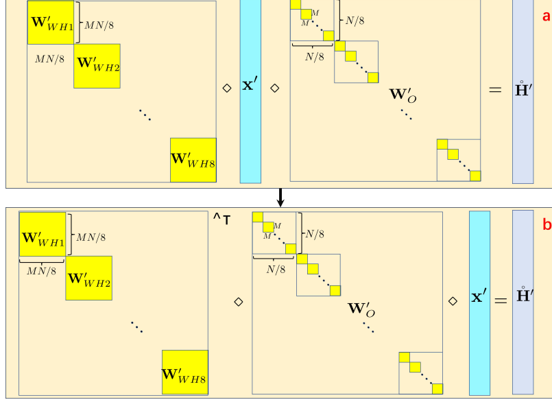
Figure 9: This figure illustrates the process of deriving the matrix-vector form corresponding to the entire multi-head attention mechanism, which is represented as \mathbf{W}_{WH}^T \diamond \mathbf{W}'_O \diamond \mathbf{x}' .
