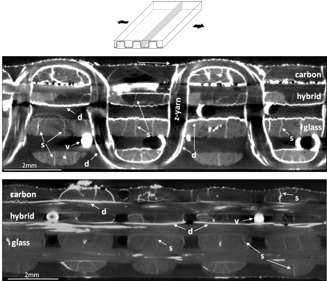
Figure 9: Tomograms of the coupon loaded in the fill direction up to 1.74% strain. (a) Transverse section perpendicular to the loading axis (b) Another transverse section perpendicular to the loading axis which contains the PE z-yarns. Glass fiber yarns appear light grey, carbon fiber yarns and matrix appear dark grey and white regions correspond to cracks or voids infiltrated by ZnI. Arrows indicate the different damage mechanisms: t tensile cracks within the fiber tows, d delamination of the fiber tows, s indicates shear cracks within the fiber tows, and v voids.
