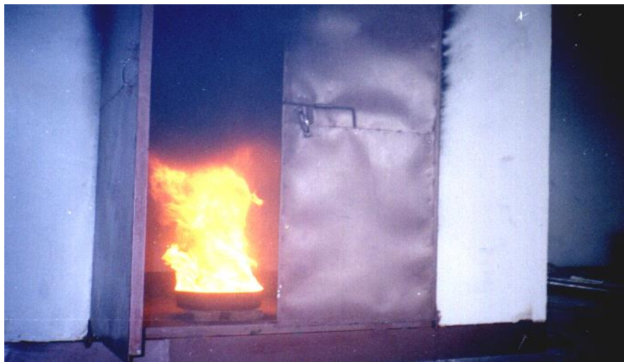
Fig. 3: A typical cabin fire test 5
