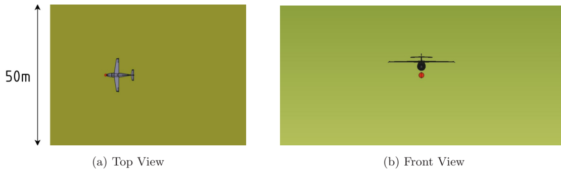
Figure 4.9: Top and Front View of Background Mesh for the Cantilever Wing Configuration
