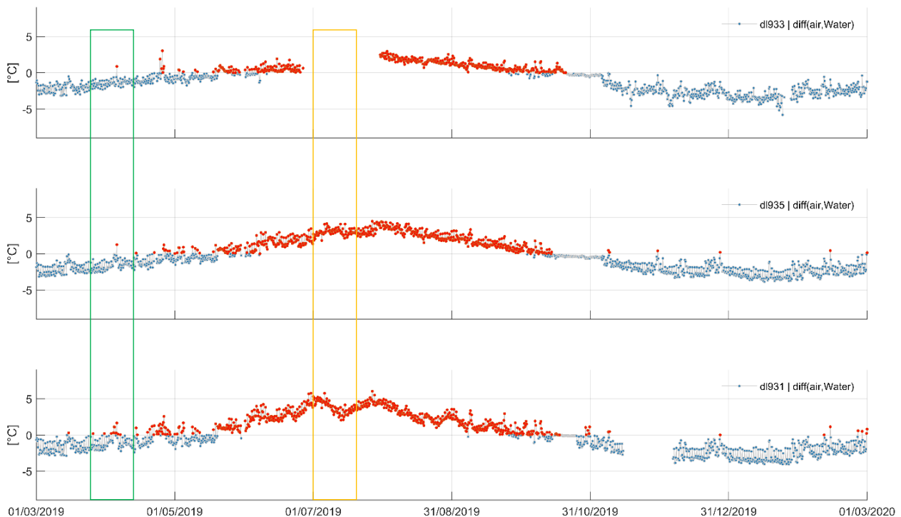
Figure 10: The difference between the sewer headspace temperature and the bulk liquid temperature observed at three specific locations in the main collector. Red dots indicate periods of evaporation (higher temperature in the headspace compared to the bulk liquid) and blue colours indicate periods of condensation (inverse temperatures). From the SI of Figuroa et al. (2022).
