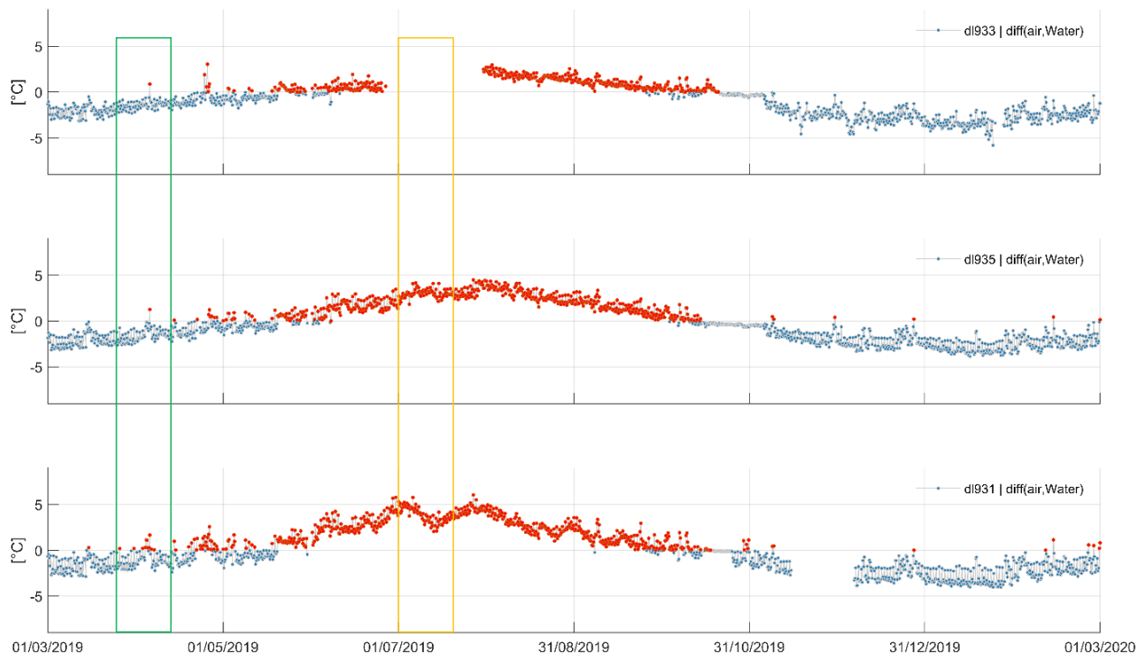
495 Figure 10: The temperature difference between the sewer headspace and the bulk liquid observed at three specific locations in the main collector. Red dots indicate periods of evaporation (higher temperature in the headspace compared to the bulk liquid) and blue colours indicate periods of condensation (inverse temperatures) (from the Supporting Information of Figuroa et al. (2022)).
