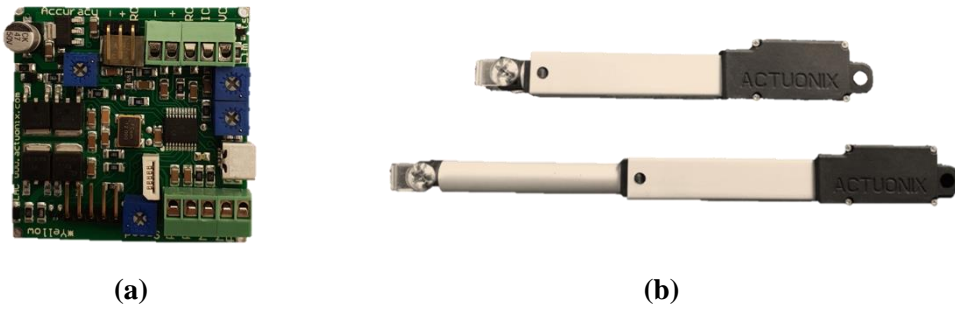
Figure 7: (a) Control board and (b) linear actuator in its fully contracted and extended states
