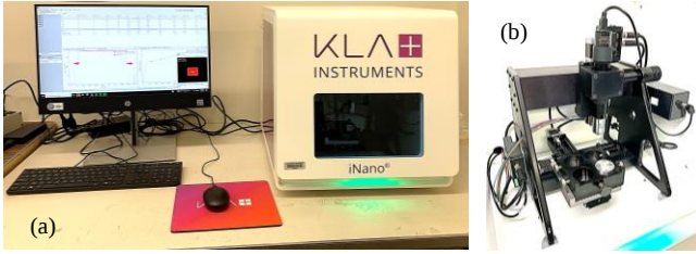
Figure 4. (a) Nanoindenter and (b) sample mounted on the holder for indentation test to find tissue properties.
