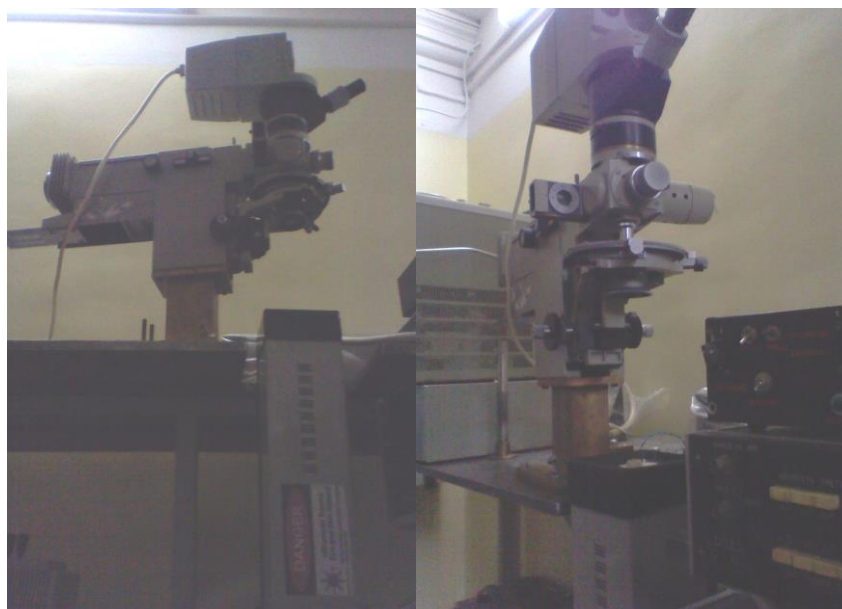
Fig. 5. Ultraviolet (micro)beam setup prototype based on nitrogen laser ILGI-503 and scanning microspectrophotometer MSPhP (Inst. En. Prob. Chem. Phys., 2016).
