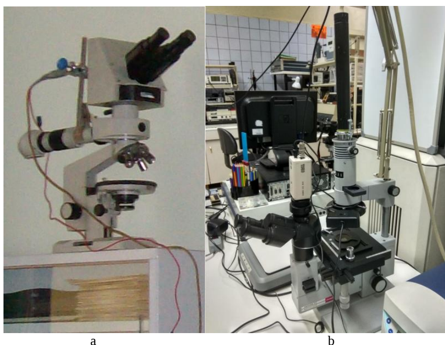
Fig. 6. Contemporary Russian compact microbeam setups for field and (auto-)mobile lab conditions: a) combined laser diode / DPSSL compact microscope for hydrobiochemical / geobiochemical and hydrobiological microbeam investigations (GEOKHI RAS, Oleg Gradov, 2010); b) HeNe laser microbeam setup based on inverted phase-contrast microscope (INEPCP RAS, Andrew Skrynnik, 2017).
