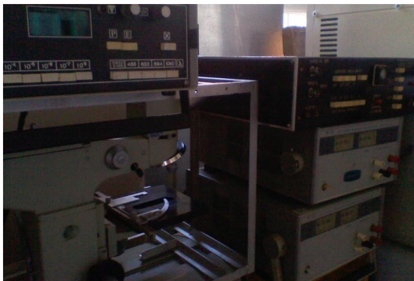
Fig. 8. Prototype of the ultraviolet microscope and ultraviolet microbeam setup in the external fields in the Faraday cage rag (based on mobile luminescence / fluorescence microscope MLD, multi-wavelength laser photometer FM-01 and photomultiplier-assisted quantometer, which also was used in the prototype UV setup on the Fig. 5). Project initiator: F. Orekhov (Gradov's Biophysical instrumentation group, 2017).
