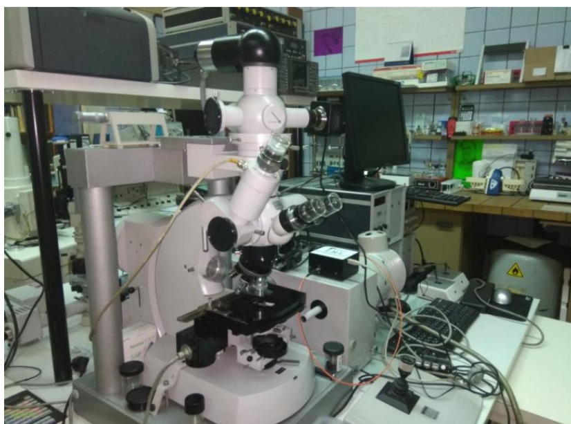
Fig. 4. Contemporary computerized version of the UV microbeam setup based on ZEISS OPTON photomicroscope with optical waveguide spectrometer, UV microspectrometer, ZEISS OPTON micromanipulator and computer-assisted data acquisition system. Semenov Institute of Chemical Physics, Gradov's multiparametric microscopy infrastructure, 2018.
