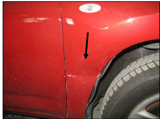
Figure 12 – Photographs of right-hand side damage to rear and front wheel arch.
