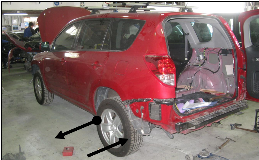
Figure 3 – Photo showing angular displacement of rear wheel (arrows show direction).
