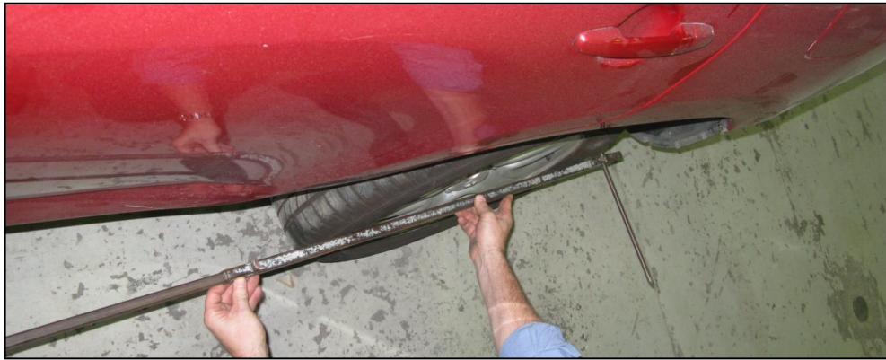
Figure 4 – Straight-edge on wheel showing outward displacement.
