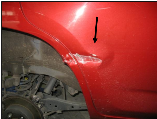
Figure 12 – Photographs of right-hand side damage to rear and front wheel arch.
