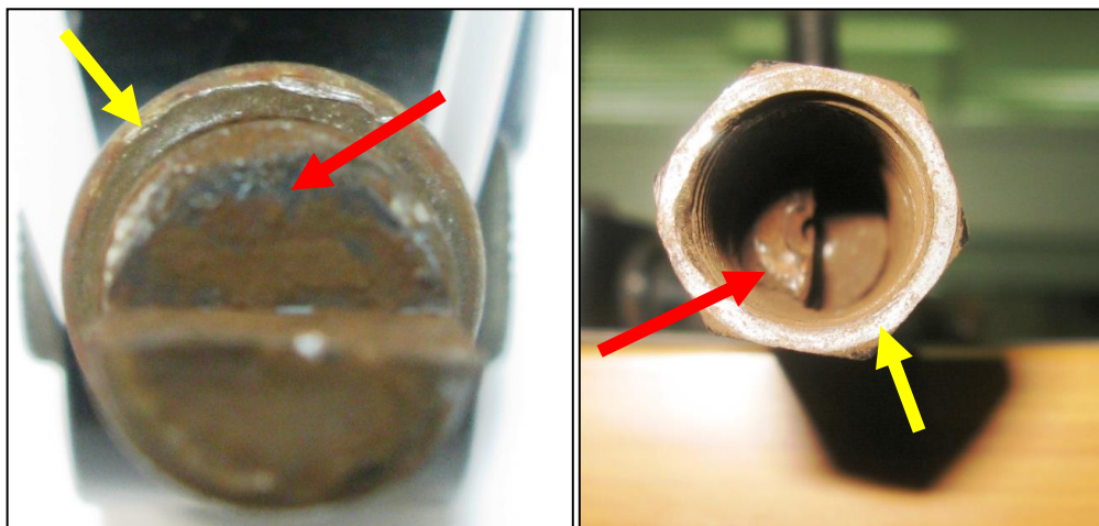
Figure 17 – End view photos of subcomponents showing burnished surfaces (colour of arrows indicates paired surfaces).
