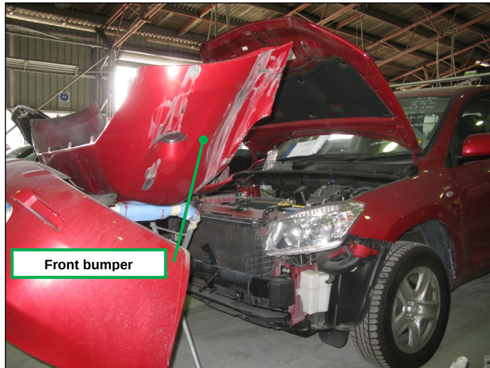
Figure 13 – Photograph of the front bumper showing damage to right-hand side. (Bumper was stored upside down).
