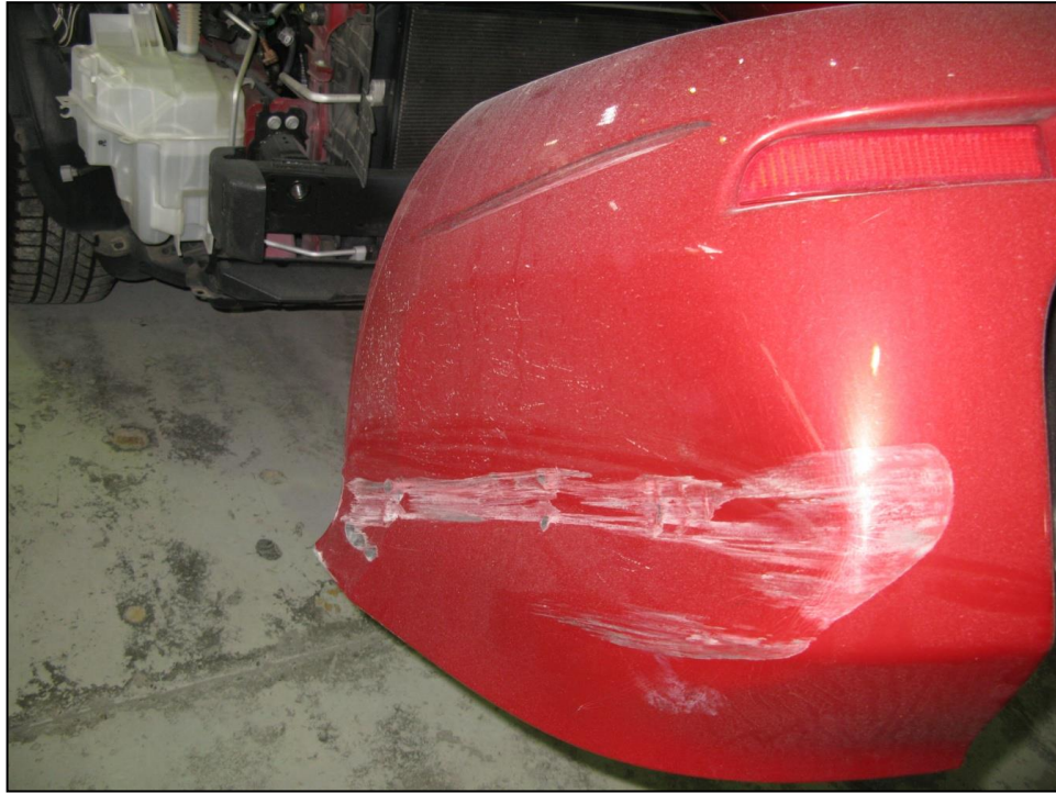
Figure 11 – Photograph of rear bumper showing damage to right-hand side. (Bumper was stored upside down)
