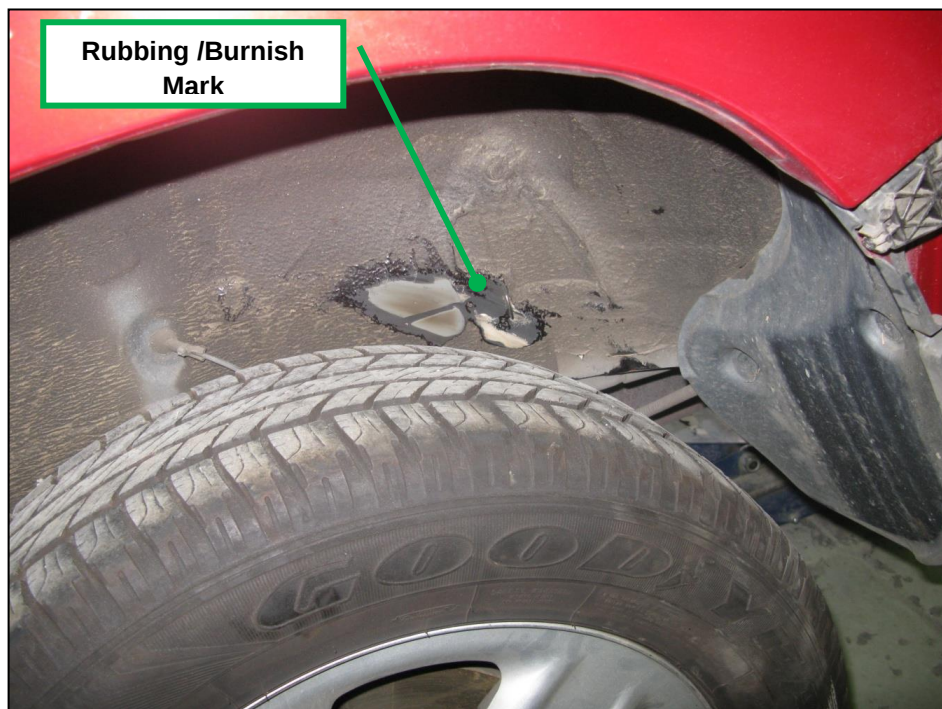
Figure 24 –Heavy rubbing mark in left-hand side rear wheel arch.
