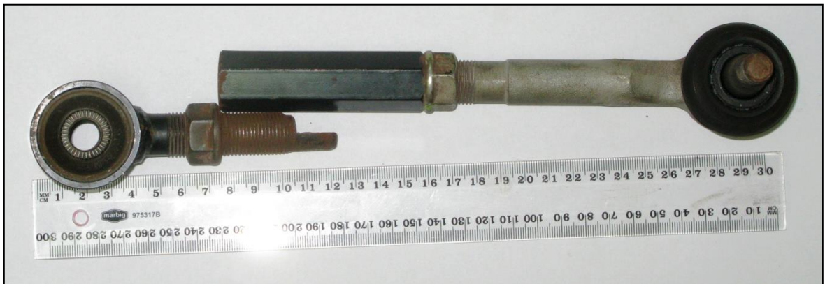
Figure 16 – Disassembled Rear Number 1 Suspension Arm into two sub components.
