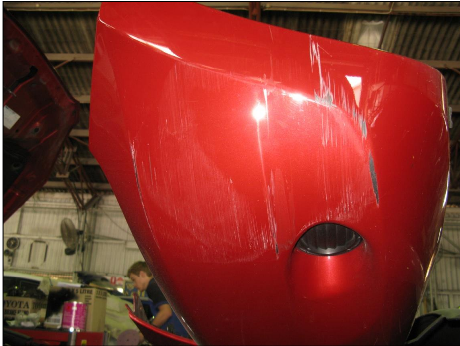
Figure 15 – Close-up photograph of the front bumper showing damage to the left hand side. (Bumper was stored upside down).
