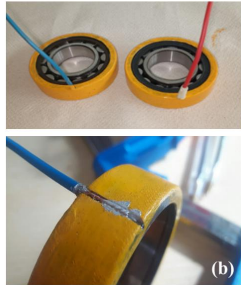
Fig. 5: (a) Electrical measurement method, (b) Fixing the wires
