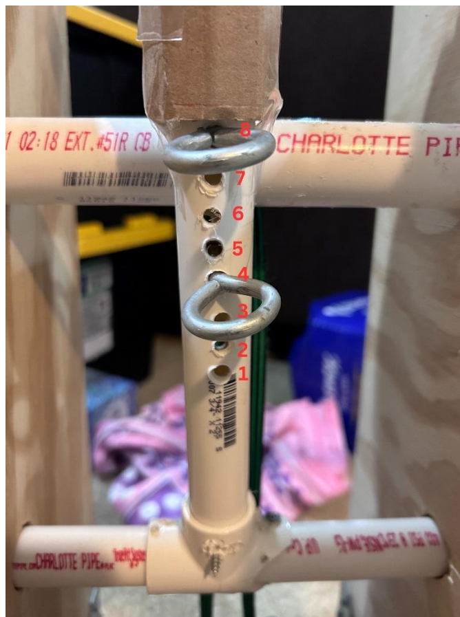
Figure 6: Arm Holes. These are the 8 small holes on the arm part of the stopping mechanism. The numbers in red are used to identify each hole. For example, this image has the arm holes set to 8 and 4. Note that the bigger number is always put first when identifying each hole.
