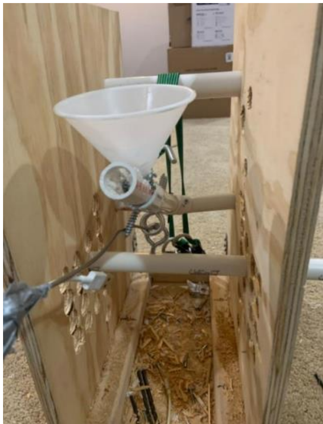
Figure 5: The Stopping Mechanism. This contraption attempted to preserve the final angle for any specific calibration of the catapult by fixing the launch angle.
