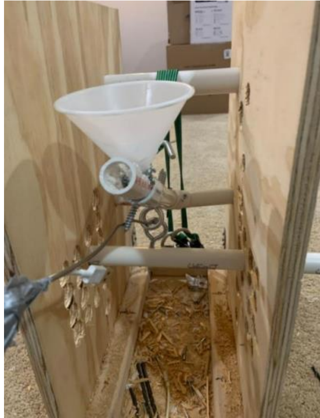
Figure 4: The Stopping Mechanism. This contraption attempted to preserve the final angle for any specific calibration of the catapult by fixing the launch angle.
