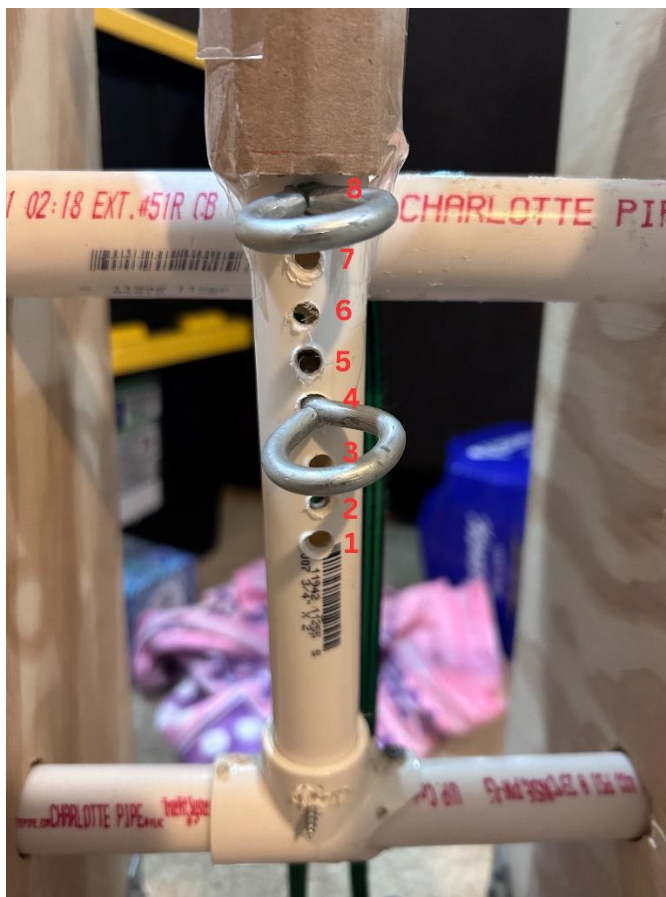
Figure 5: Arm Holes. These are the 8 small holes on the arm part of the stopping mechanism. The numbers in red are used to identify each hole. For example, this image has the arm holes set to 8 and 4. Note that the bigger number is always put first when identifying each hole.
