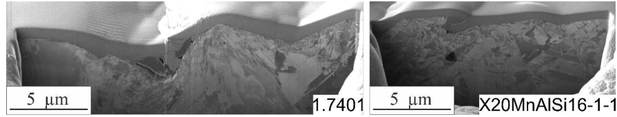
Fig. 12.5: Near surface layer after modified lapping process.
