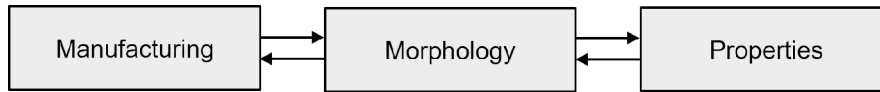
Fig. 1.1: Scheme of Manufacturing-Morphology-Property Relationships (MMPs) for mechanical components as they are studied in the present book. The arrows indicate the relations, which lead either from the manufacturing to the properties or in the reverse direction, from desired properties to a suitable manufacturing process.
