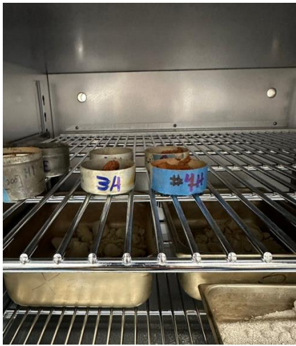
Figure 13. Soil Moisture Content Test. Oven drying sample.
