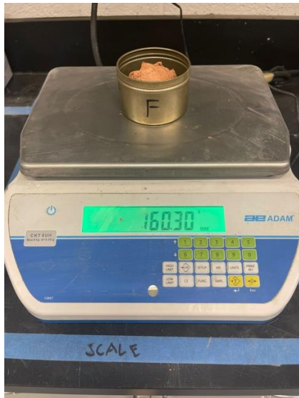
Figure 12. Soil Moisture Content Test. Initial measure of soil moisture content.
