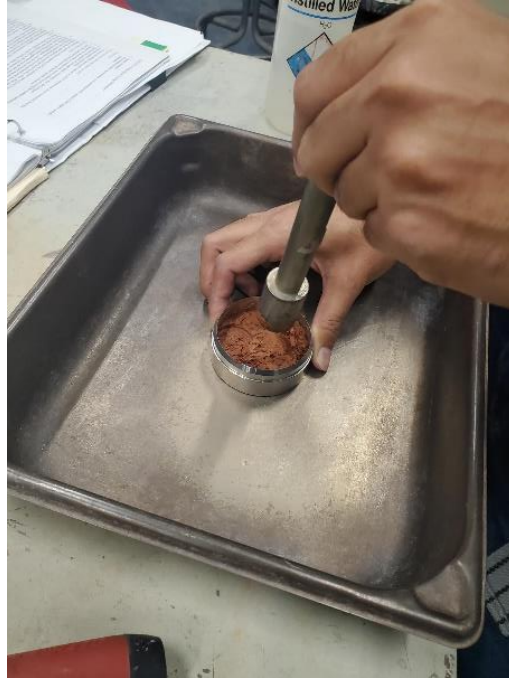
Figure 3. Preparation of the clay sample in the consolidation ring.
