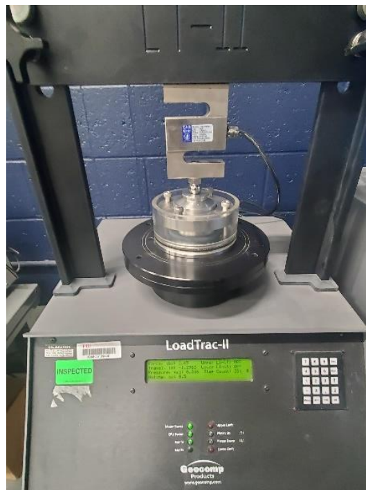
Figure 4. Sample placed on the LoadTrac-II device with applied load.
