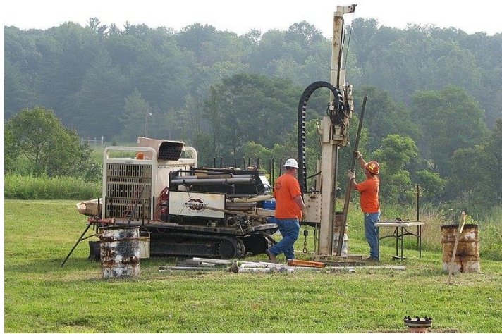
Figure 9. Soil Samples Removal by Augers. Public Domain Media.
