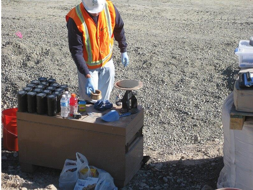
Figure 14. Flow test for underground Grout. Public Domain Media.
