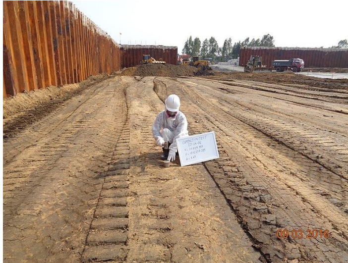
Figure 4. Compaction Test of Soil Sediment. Public Domain Media.
