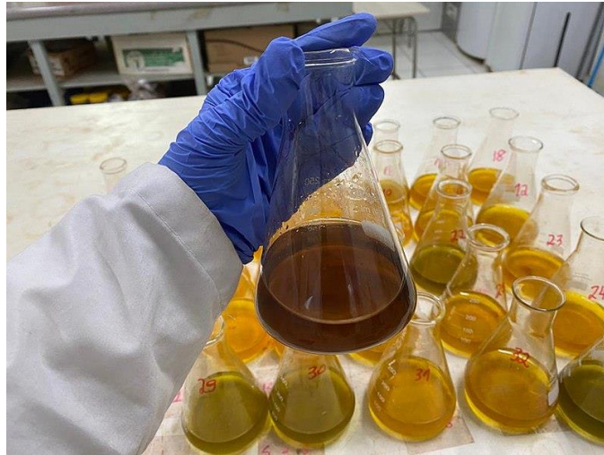
Figure 6. Soil Analysis by Titration. Public Domain Media.
