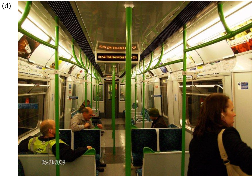
1 2 Figure 6 Three Hypothetical Forty-Four Seater Subway Car Layouts: (a) This traditional layout might cause 3 crowding around the door areas and contains 12 undesirable “middle” seats; (b) This revised layout has the same 4 seated capacity and the same standing room, but may have higher effective capacity due to better space 5 utilization; (c) This non-homogenous design offers a choice in seating layouts, allowing longer-distance 6 passengers to gravitate towards commuter-style seats at car ends, and short-distance riders to stand in the 7 middle zone with no seats; (d) London District Line’s D78 stock has mixed seating layouts within a single car.
