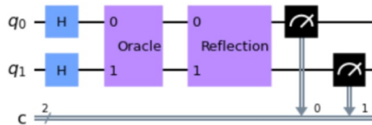
Figure 5: Quantum Circuit Representation of Grover's algorithm
