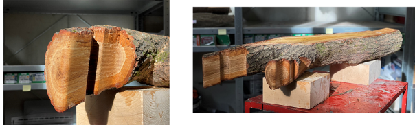
Figure 22: Structural connection: Photo of a construction element from an oak specimen, depicting the position of the contact faces of the joint, considering the central line of the tree’s growth.
