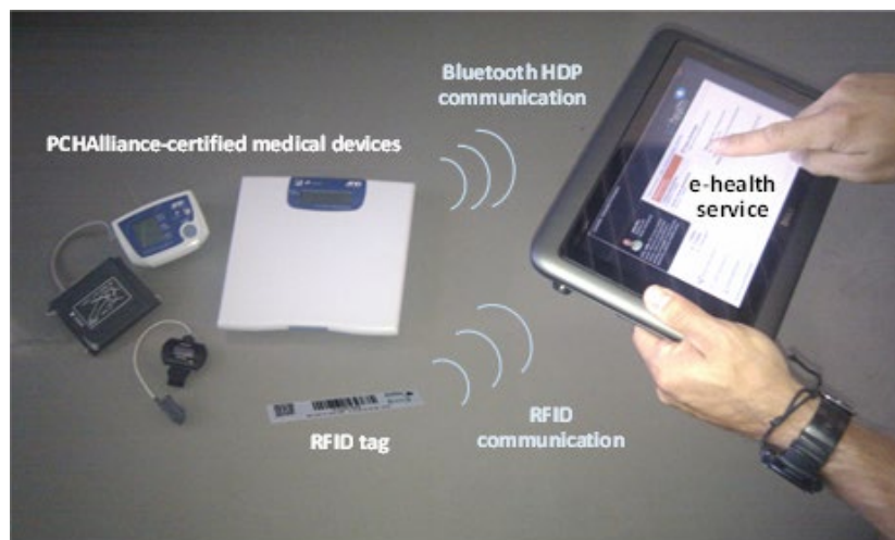
Fig 5. ISO/IEEE 11073-PHD e-health solution with PCH Alliance-certified devices over Bluetooth HDP and multiuser identification through RFID technologies
