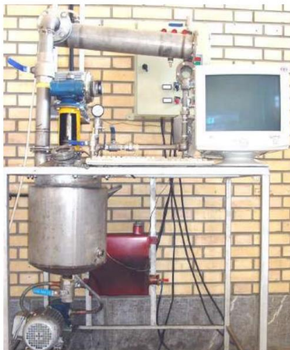
Fig. 5. 10 Liters Pilot plant for chemical recycling of PET
