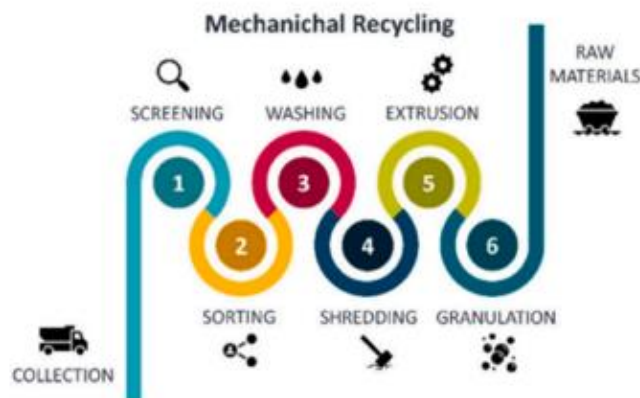
Steps of mechanical recycling of plastics [4].
