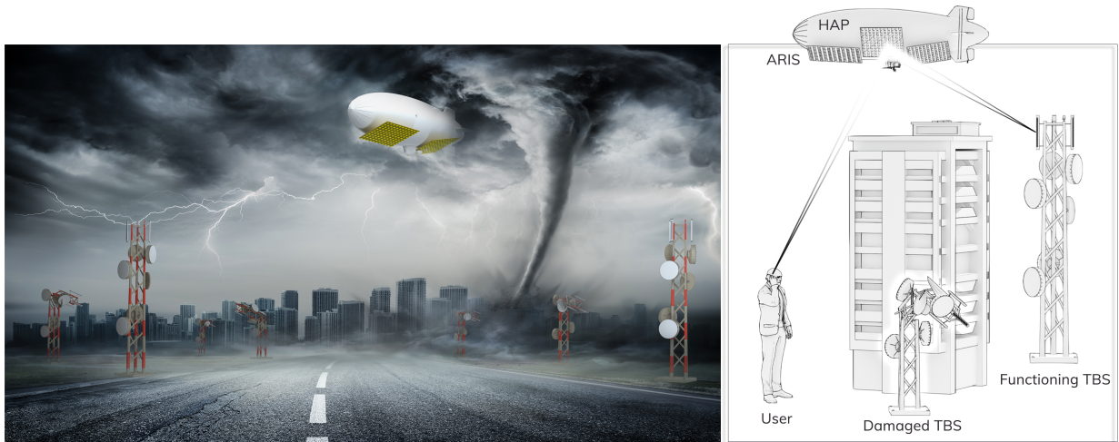
Fig. 1. System figure: ARISs can be deployed in post-disaster scenarios to improve the quality of the communication links between users and surviving TBSs.
