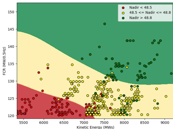
Figure 2: Overview of dynamic analysis of multiple operating points to the loss of largest infeed
