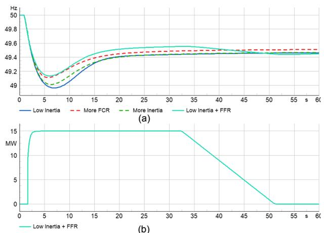
Figure 1: (a) Frequency response after loss of generation, and (b) FFR response
