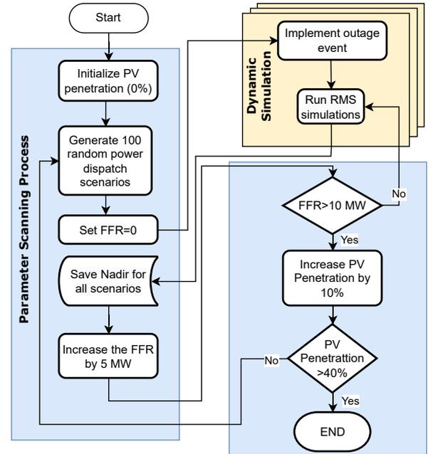
Figure 5: Flowchart of proposed investigation algorithm
