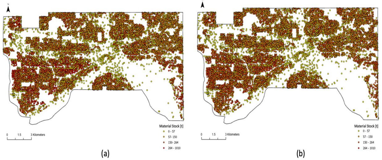
Figure 7: Total Material Stocks Map for Test Set in St. Paul. Point markers represent MS of corresponding parcels. The ground truth MS is presented in (a) and the predicted MS is shown in (b).
