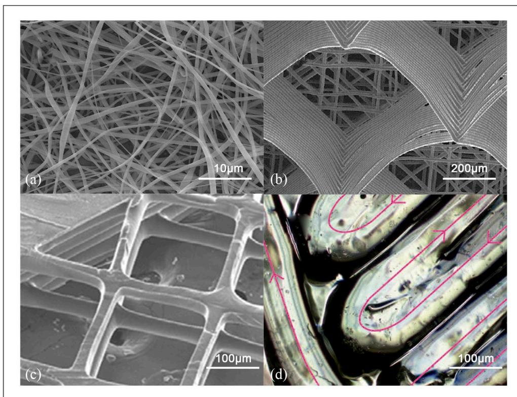
**Figure 5.** Different 3D printed structures achievable by: (a) Electrospinning. (b) Melt electro-writing. (c) Digital light processing. (d) 3D-bioprinting. Illustrations adapted with permission from Bhullar et al.,<sup>56</sup> Castilho et al.,<sup>53</sup> Soman et al.,<sup>96</sup> and Pourchet et al.,<sup>97</sup> respectively.
