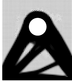
Fig. 7: Modified benchmark with adapting contact normal directions.
