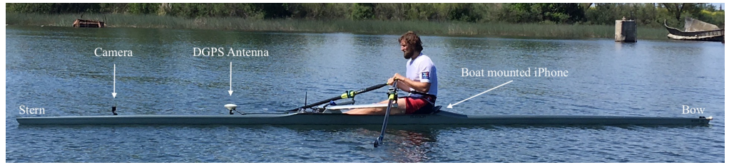
Fig 7. Sensor locations during the elite trials.
