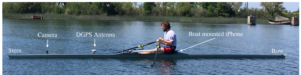
Fig 7. Sensor locations during elite trials.
