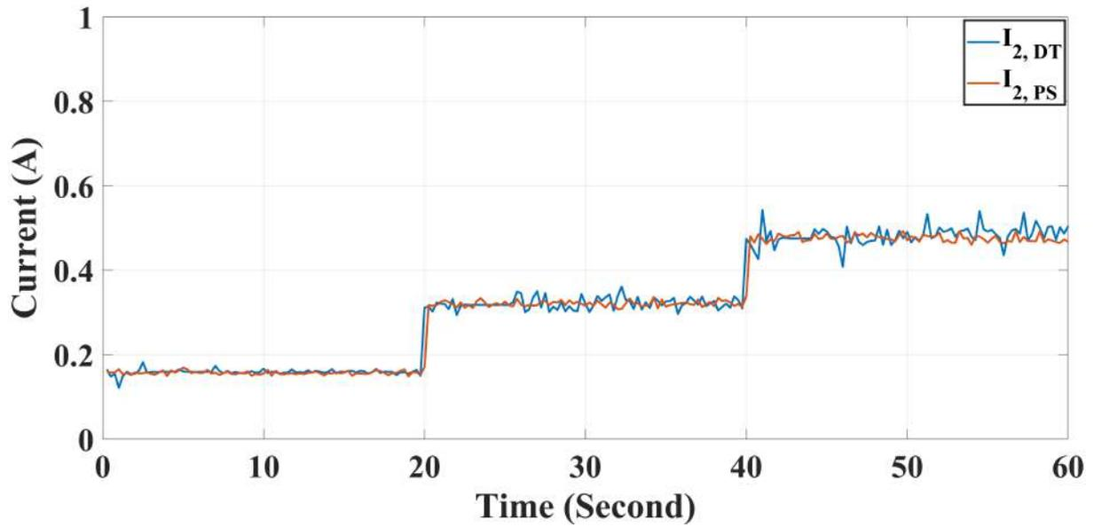
Figure 16: DT model and PS agent buck 2 current comparison in assessment test I
