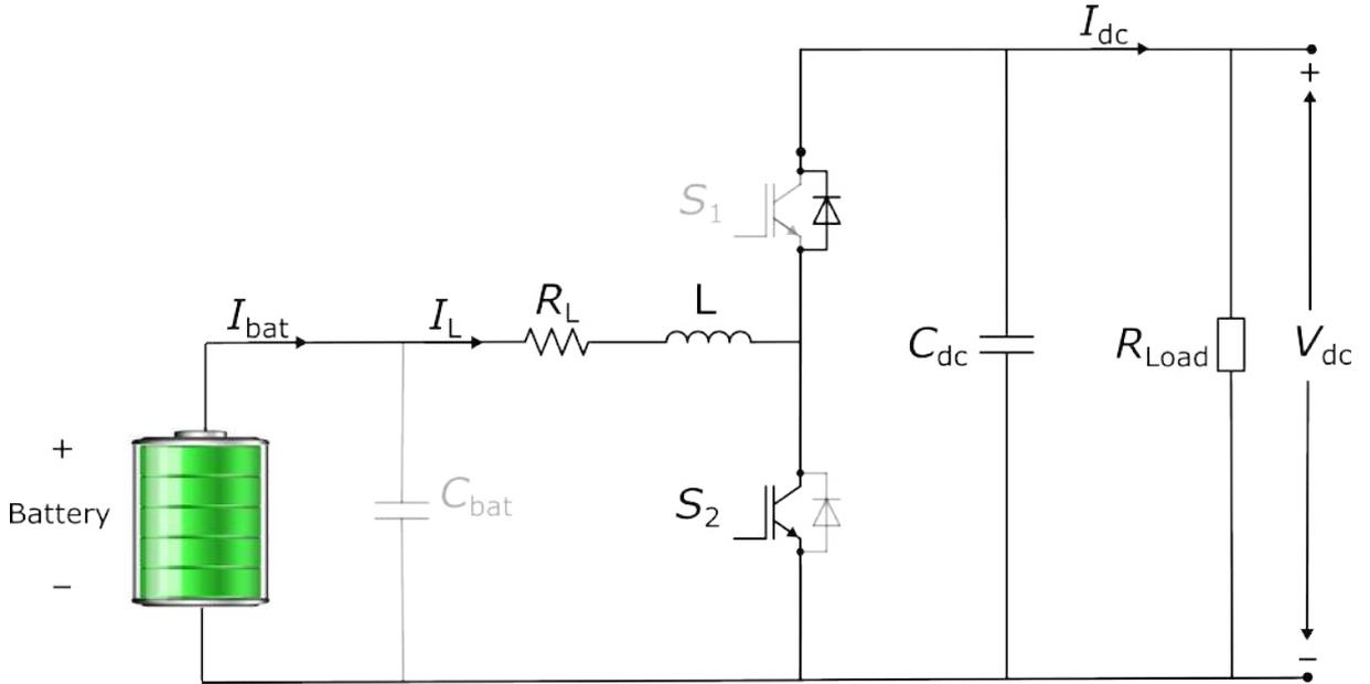
Figure 8: Configuration of Bi-directional buck-boost Converter Under Discharging Modes
