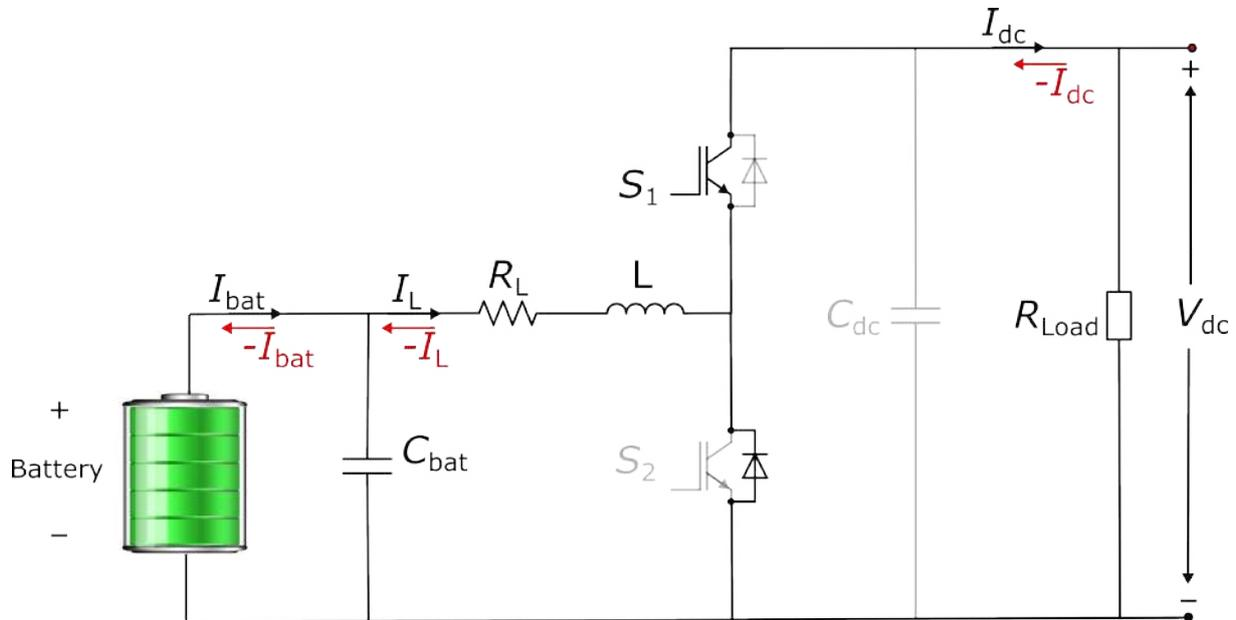
Figure 7: Configuration of Bi-directional buck-boost Under Charging Modes
