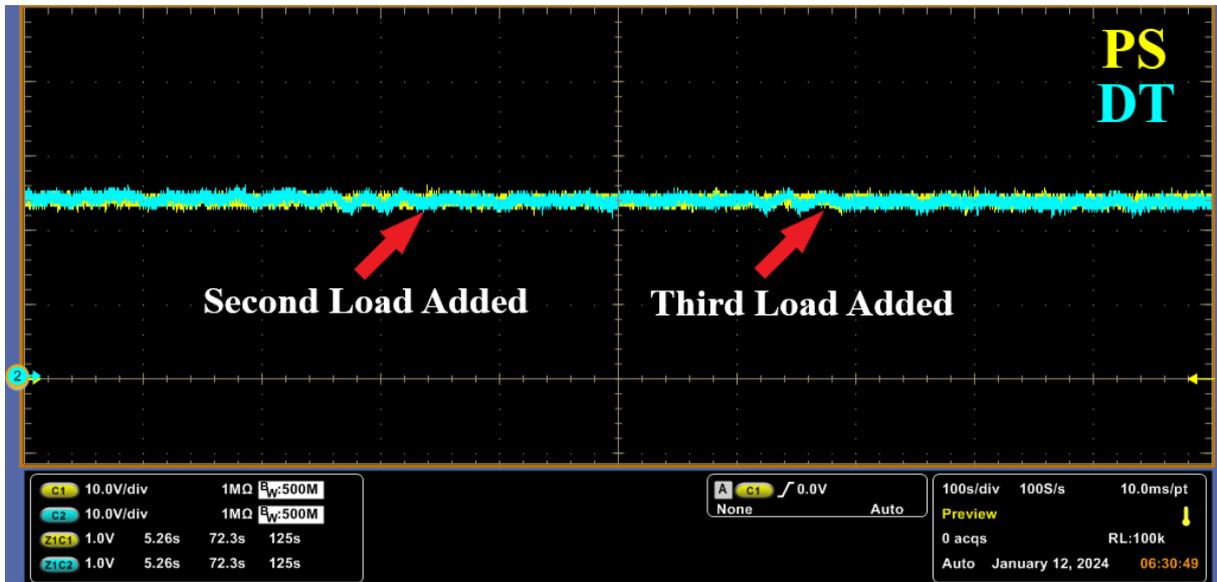
Figure 19: DT model and PS voltage comparison from the oscilloscope in assessment test II
