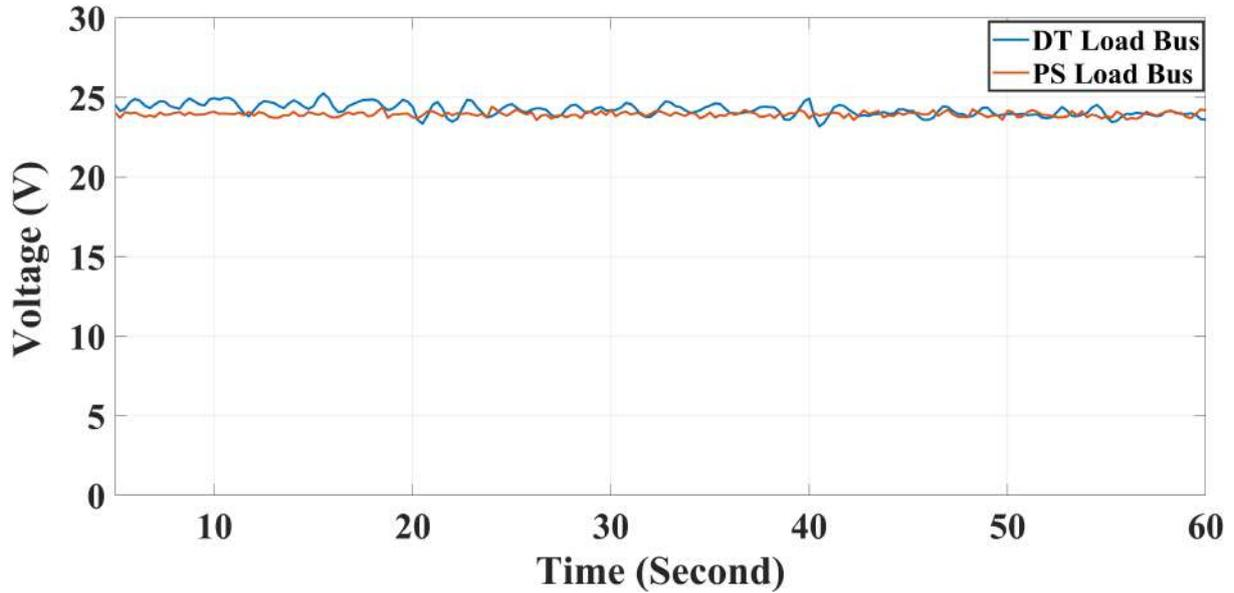
Figure 18: DT model and PS voltage comparison from HMI in assessment test II
