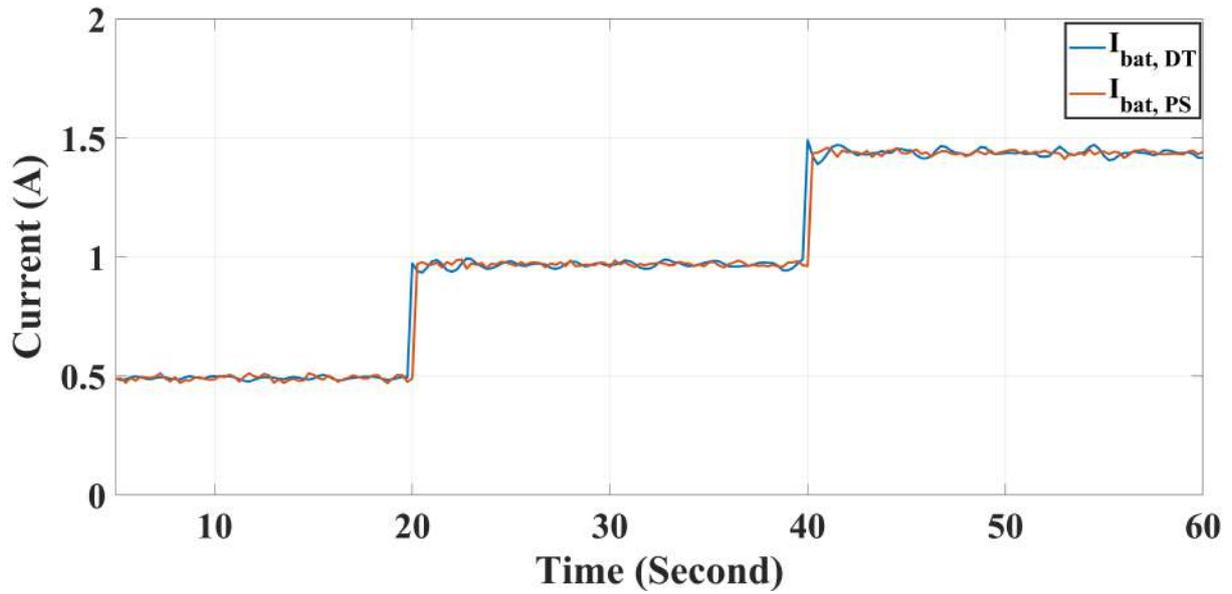
Figure 20: DT model and PS current comparison in assessment test II
