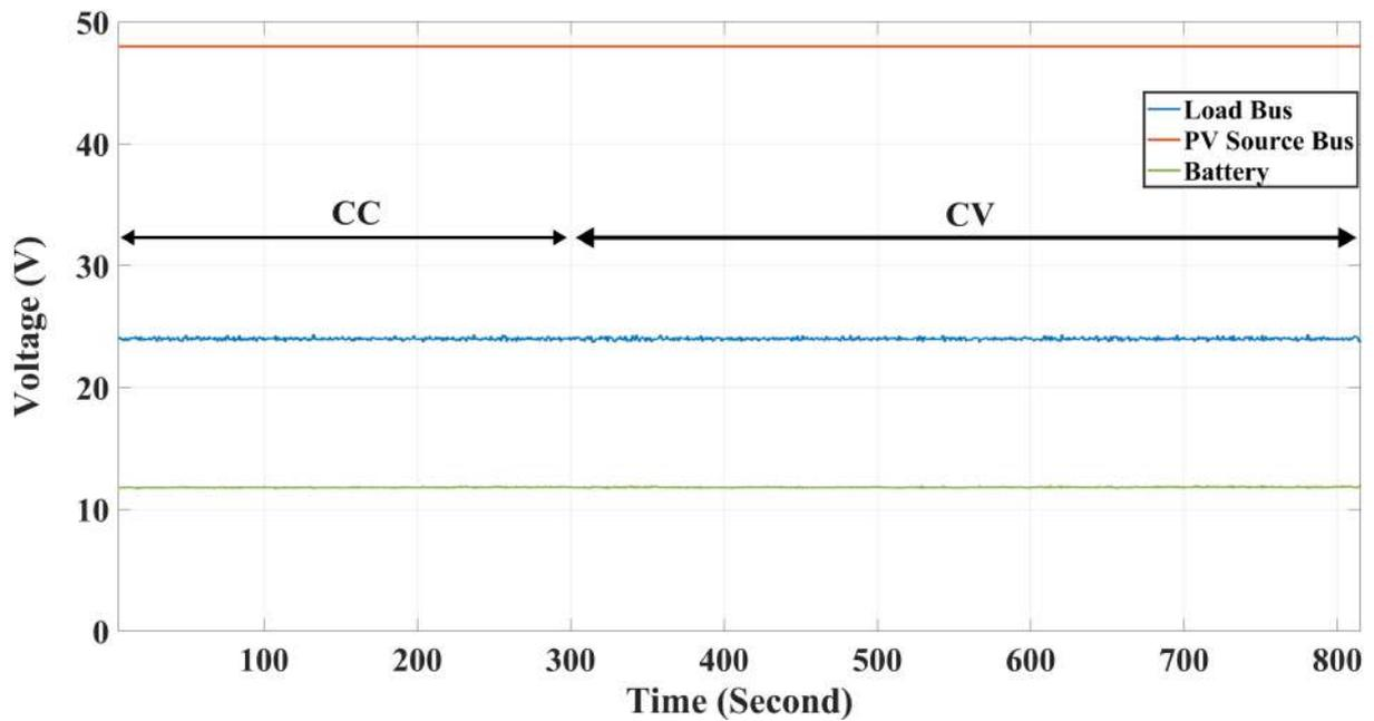
Figure 25: Voltage waveforms in emergency support charging scenario II
