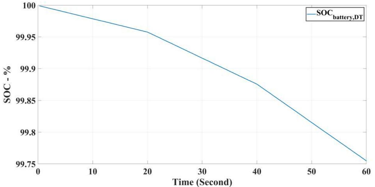
Figure 21: The battery SOC during discharging in assessment test II
