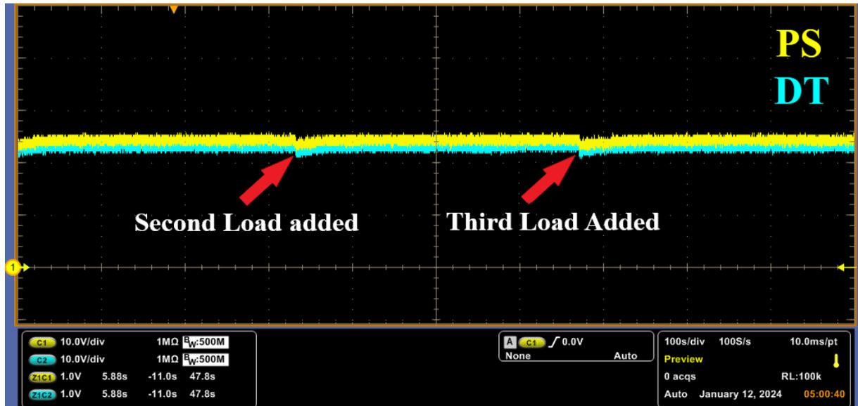
Figure 13: DT model and PS voltage comparison from the oscilloscope in assessment test I
