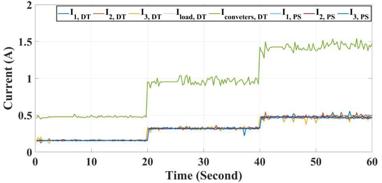
Figure 14: DT model and PS all currents comparison in assessment test I
