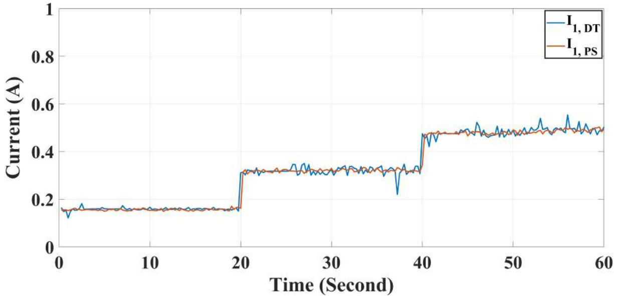
Figure 15: DT model and PS agent buck 1 current comparison in assessment test I
