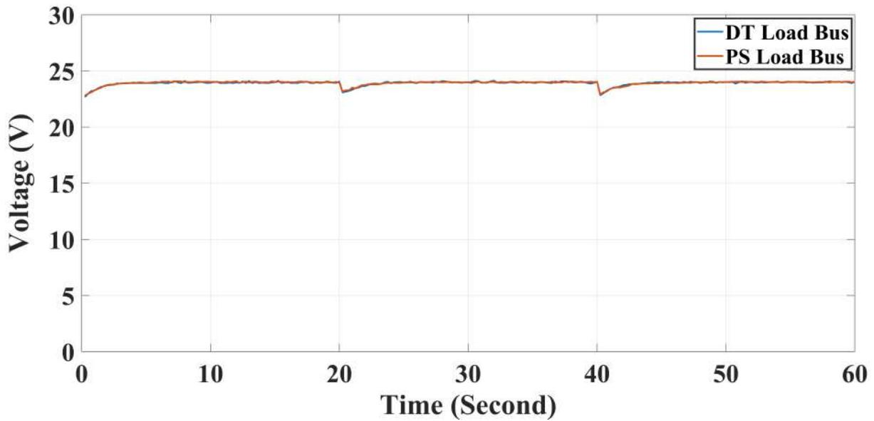
Figure 12: DT model and PS voltage comparison from the HMI in assessment test I
