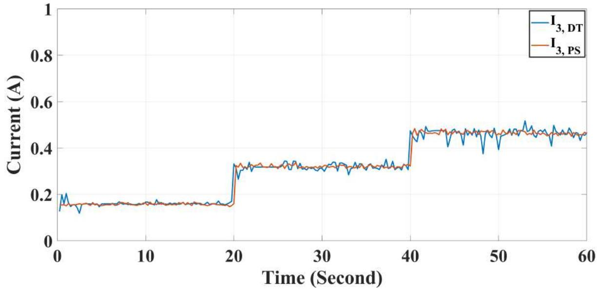
Figure 17: DT model and PS agent buck 3 current comparison in assessment test I
