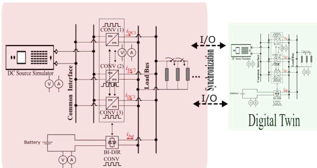
Figure 9: DC microgrid live DT
