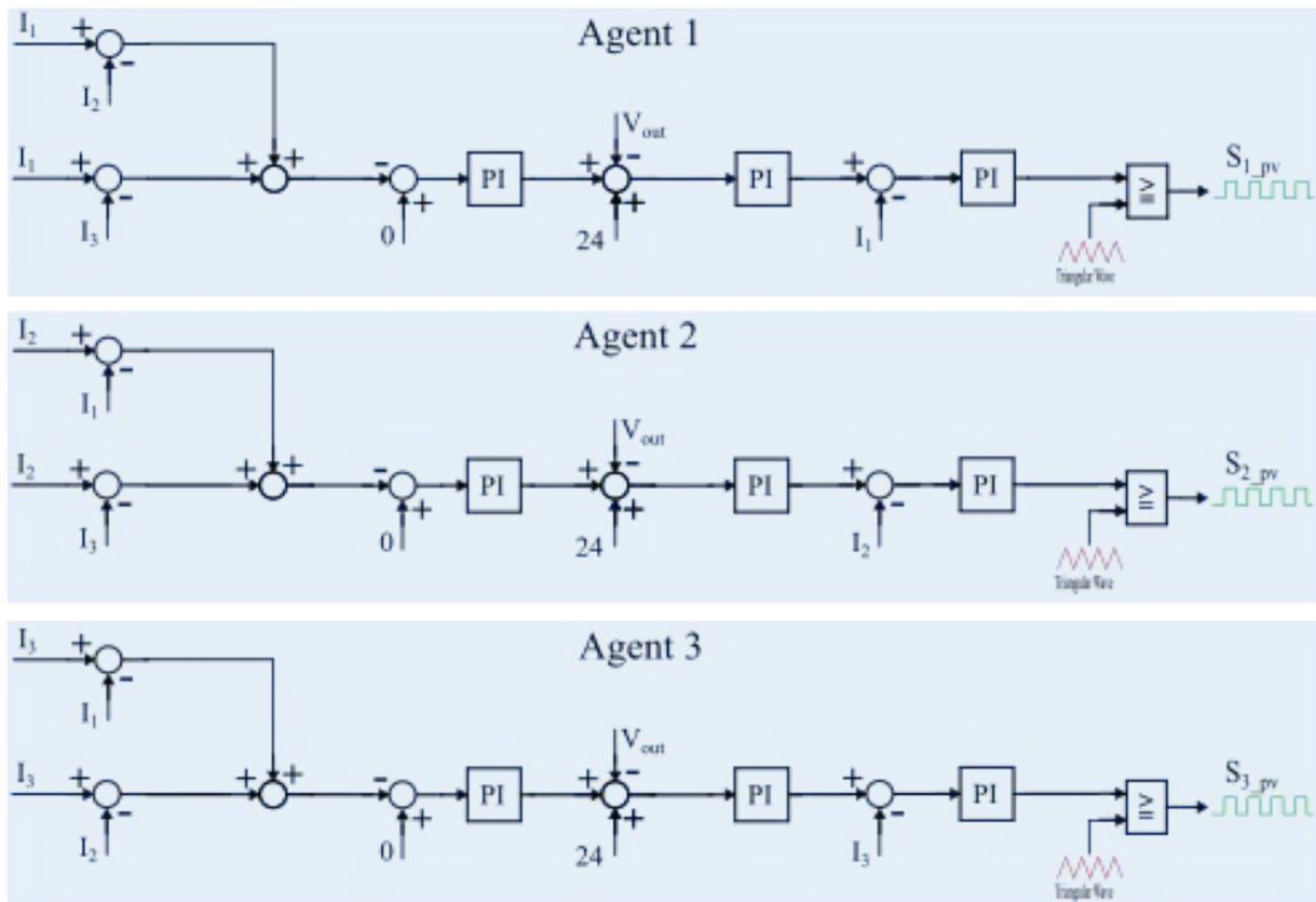
Figure 5: Current Sharing Control Diagram
