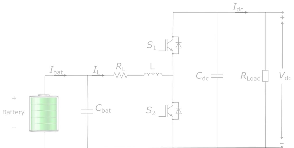
Figure 6: Configuration of Bi-directional buck-boost Under Normal Operation
