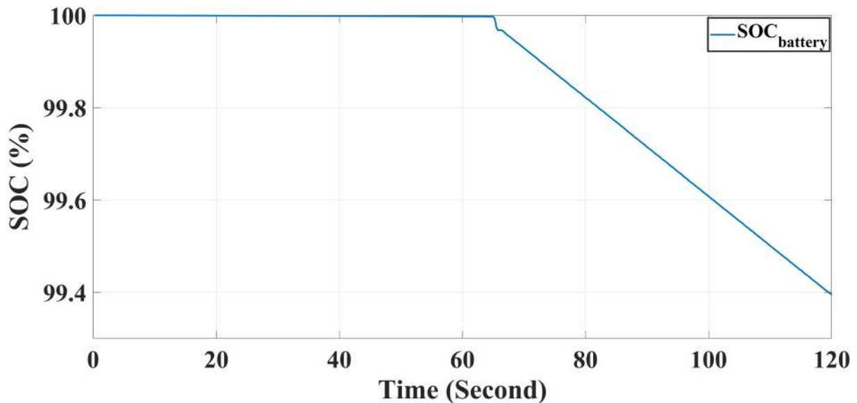
Figure 24: Battery SOC in emergency support discharging scenario I
