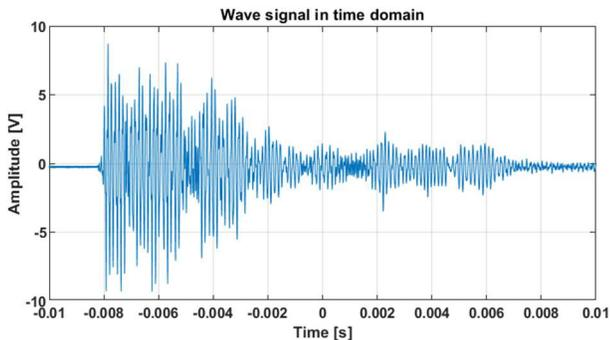
Fig. 4. Signals detected during the measurements (intact insulator).
