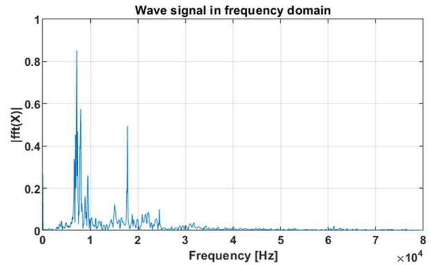
Fig. 5. Spectrum of the signal (intact insulator).
