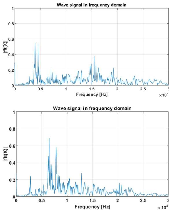
Fig. 7. – Spectra of the signal (intact insulator).
